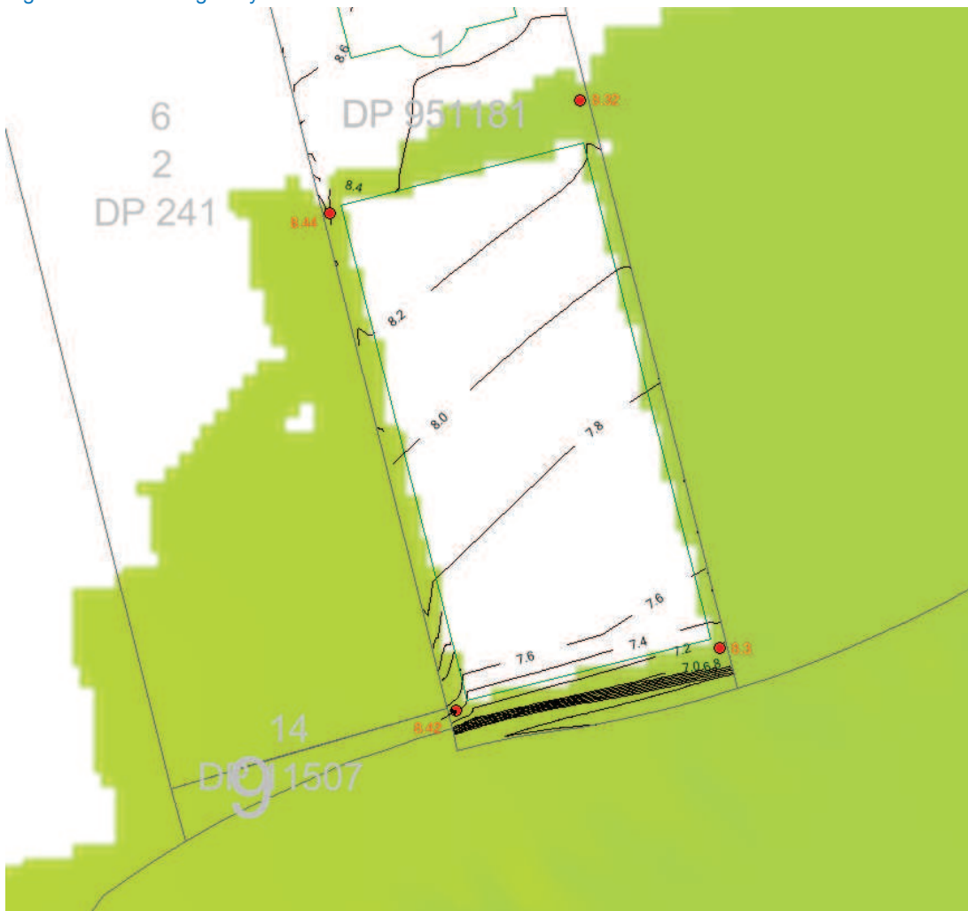
Figure B.1: Existing 100yr flood extents
